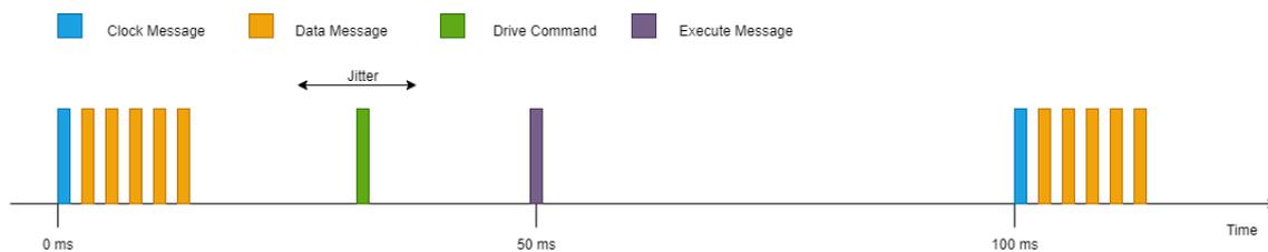
**Figure 8.3:** Can time diagram
