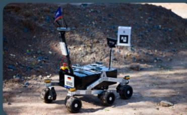
For the first time, we have to work with volume, current and centre of gravity budgets. The aim is to extract, analyse and transport a 100 gram sample without mixing from a depth of >300 mm from simulated Martian regolith. The DSD module will compete together with ORTHOS at the international European Rover Challenge in Krakow.
